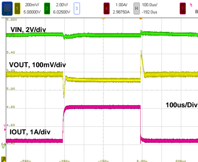
Figure 27. Load Transient, 0.2A-2A-0.2A
